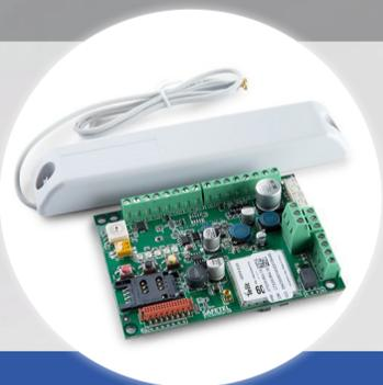
The Airborne DC range combines many types of alarms and transmits them digitally via the mobile network to the right alarm receiver. It utilises both a PCB antenna and the LPW-BC3G-26 from Panorama Antennas
